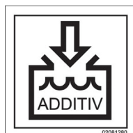
Water tank inlet of additive sprinkling
